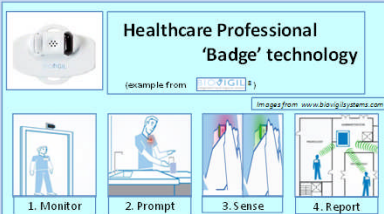
Figure 5: Here a Healthcare Professional wears a badge which senses location, reminding the wearer of the need to perform Hand Hygiene by glowing RED , changing colour to GREEN once hands have been cleaned using substance containing alcohol, which is sensed as hands are held up to badge. Instant visual feedback provided to peers and Patients, data is stored for analysis.
